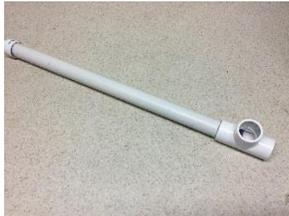
**Step 6** – *Attaching Tee Joints to Mid-Section*
