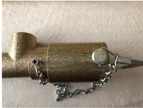
*(Couplings, Tee Joint, Zinc Chain, Screw, Wire Square Lock Pin, and painted)*
